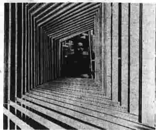
ALUMINUM STORM WINDOWS can reduce heat loss through the windows as much as 40 percent because they create an insulating air space. Worker tightens screws on frames which have multiple tracks to make both storm sash and screens self-storing. Photo courtesy: the Aluminum Association.
